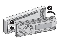
Face Plate Removing/Mounting
